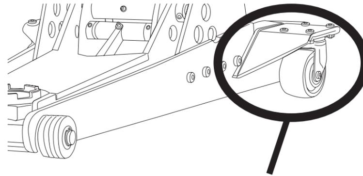
Make sure caster brackets with pre-mounted rear casters are on securely and facing in the correct direction. See diagram above for orientation
